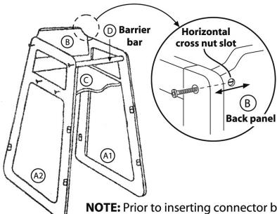
**NOTE:** Prior to inserting connector bolts into the panels, make sure that the cross nut slot stays horizontal to allow proper insertion.
